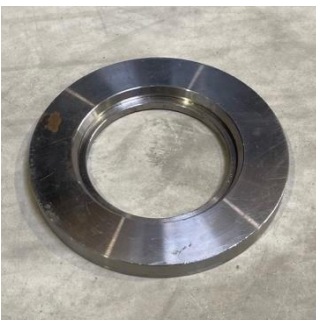
702019 Draw plate for Ø 115 mm Complete diameter 160 mm Diameter groove 115 mm Passage 103 mm For pulling the liner while the protective piping remains in the ground
